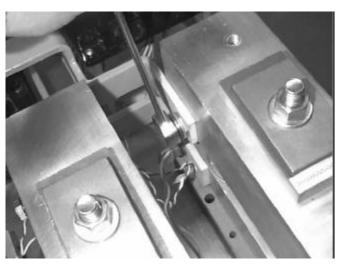
Figure 18. Removing the busbar mounting bolt.
